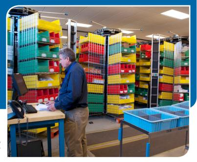
Three 52 foot long horizontal carousels with pick to light technology and FastPic order processing software manage all low units of measure inventory.
